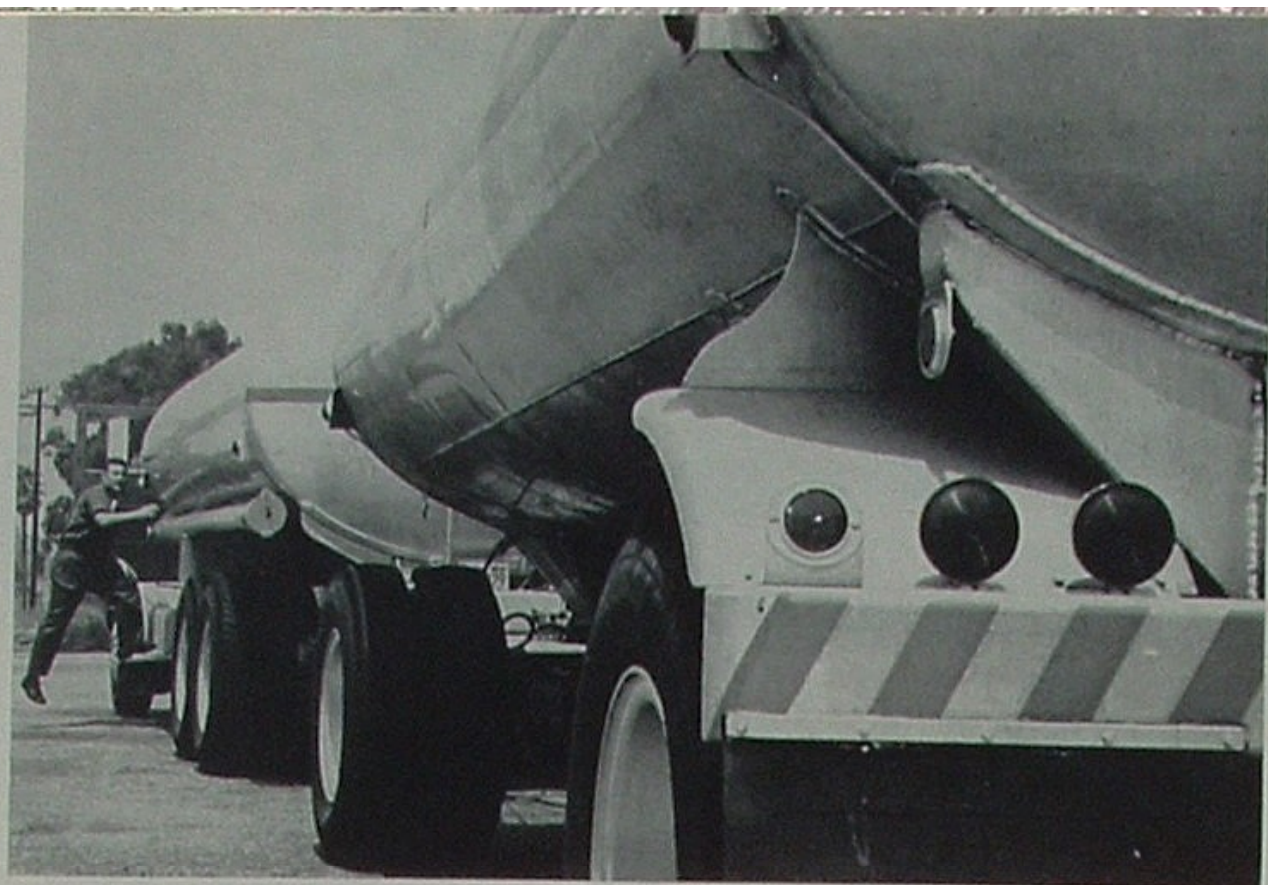
John's 9,000-gallon truck-and-trailer owes its increased carrying capacity to light metals and removal of meters.
