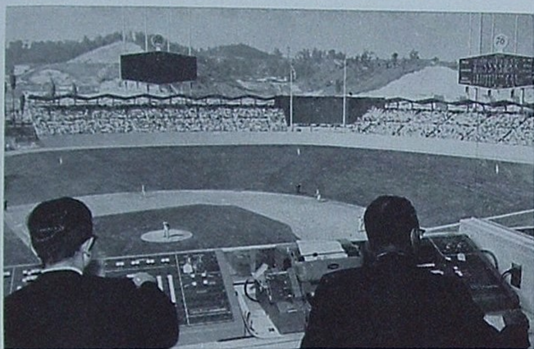
The "Finest" scoreboards in baseball are operated by remote control from the press section. Typewritten messages appear under sign at left.
