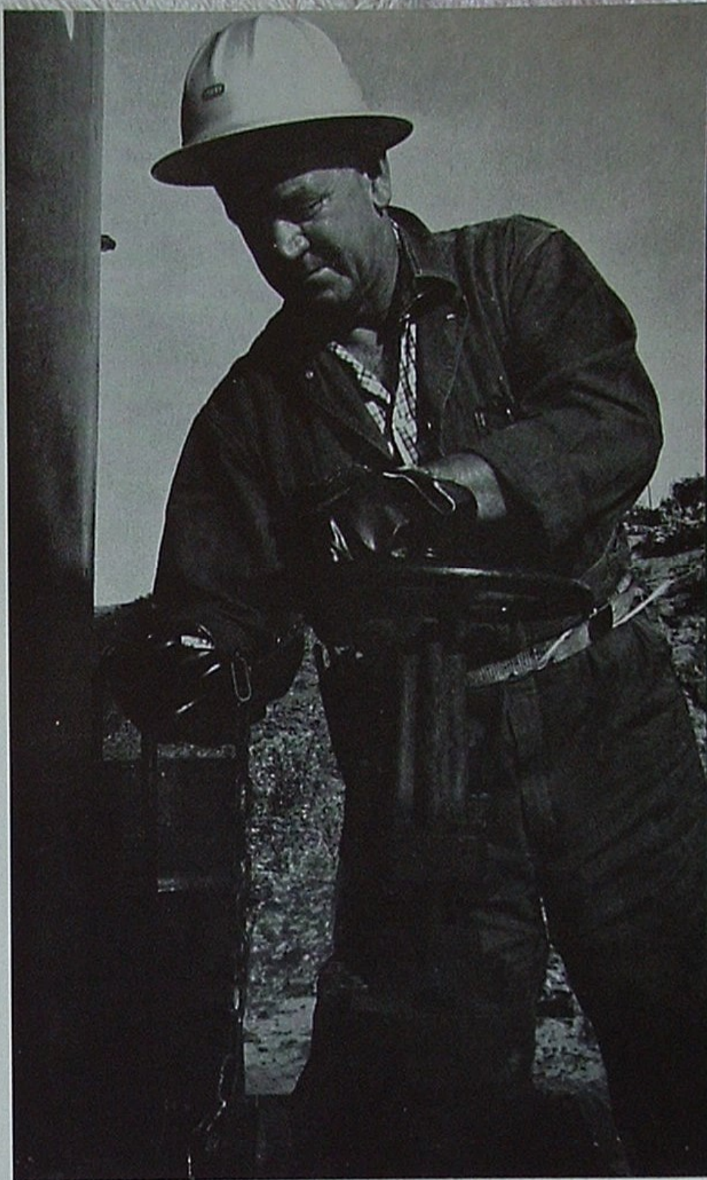
Gauger Harold Martinson chains and seals valve on tank. No oil can move from tank until he breaks the seal. He's the measuring man, responsible for every drop of oil that flows into Union Oil's pipeline from his coastal district.
