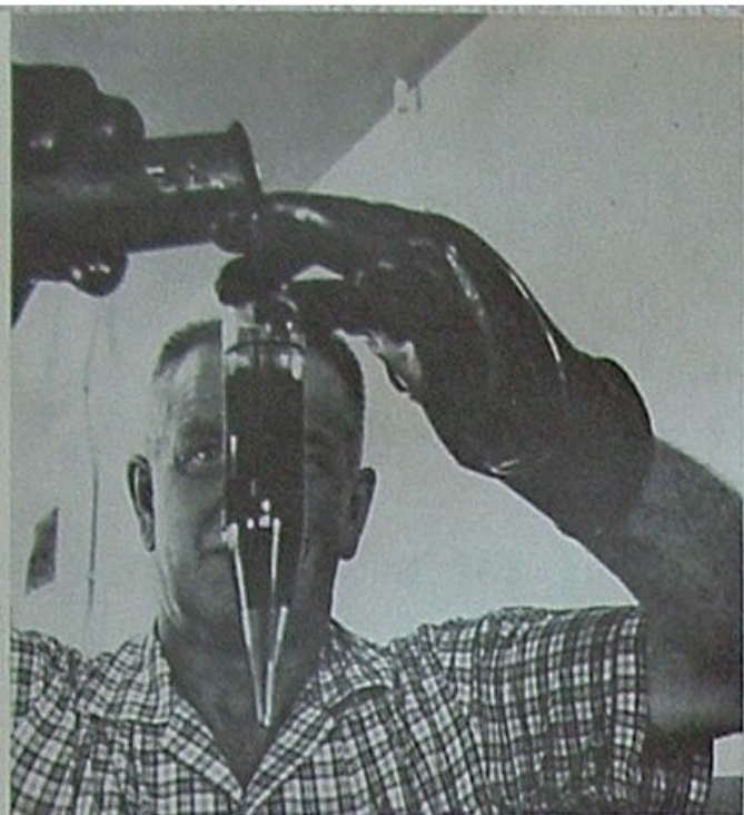
Crude oil usually contains some water; so to be sure how much of the crude he gauged is pure oil, Martinson tests a sample in the field laboratory.
