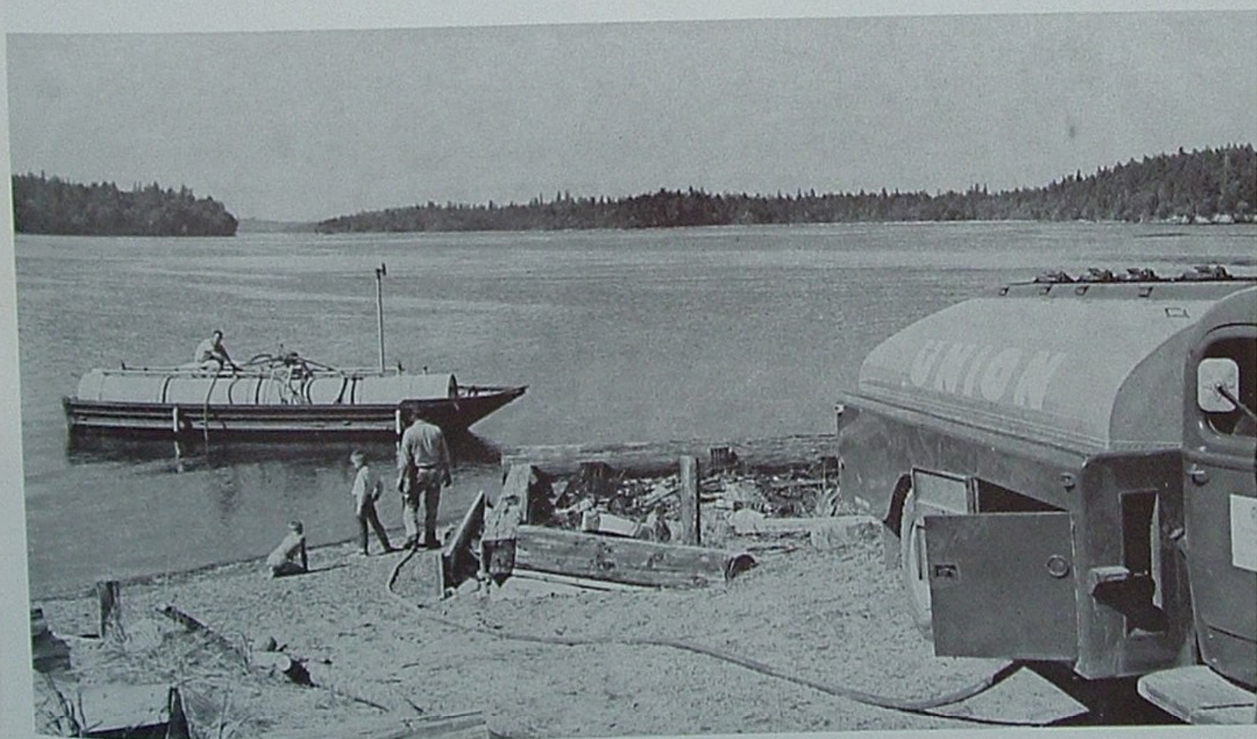
The problem of petroleum supply is solved by a 2,000-gallon tankboat seen receiving at Olympia before being towed to the sales site.
