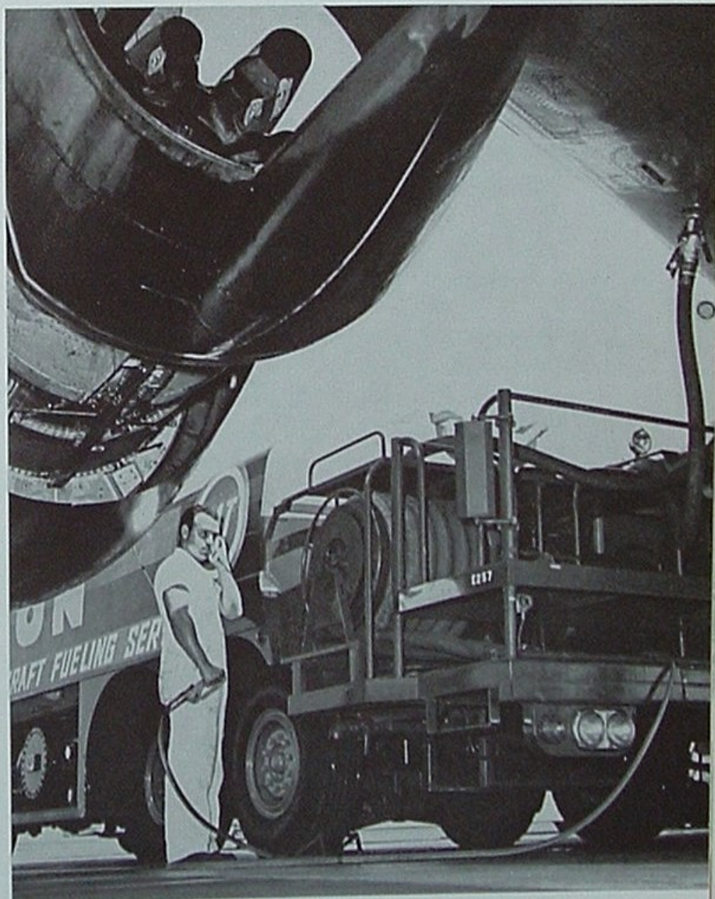
The Lockheed refueler trucks in use at both airports can load in tandem at 1200 gallons a minute. The operator, with control valve in hand, contacts jet's engineer by telephone.
