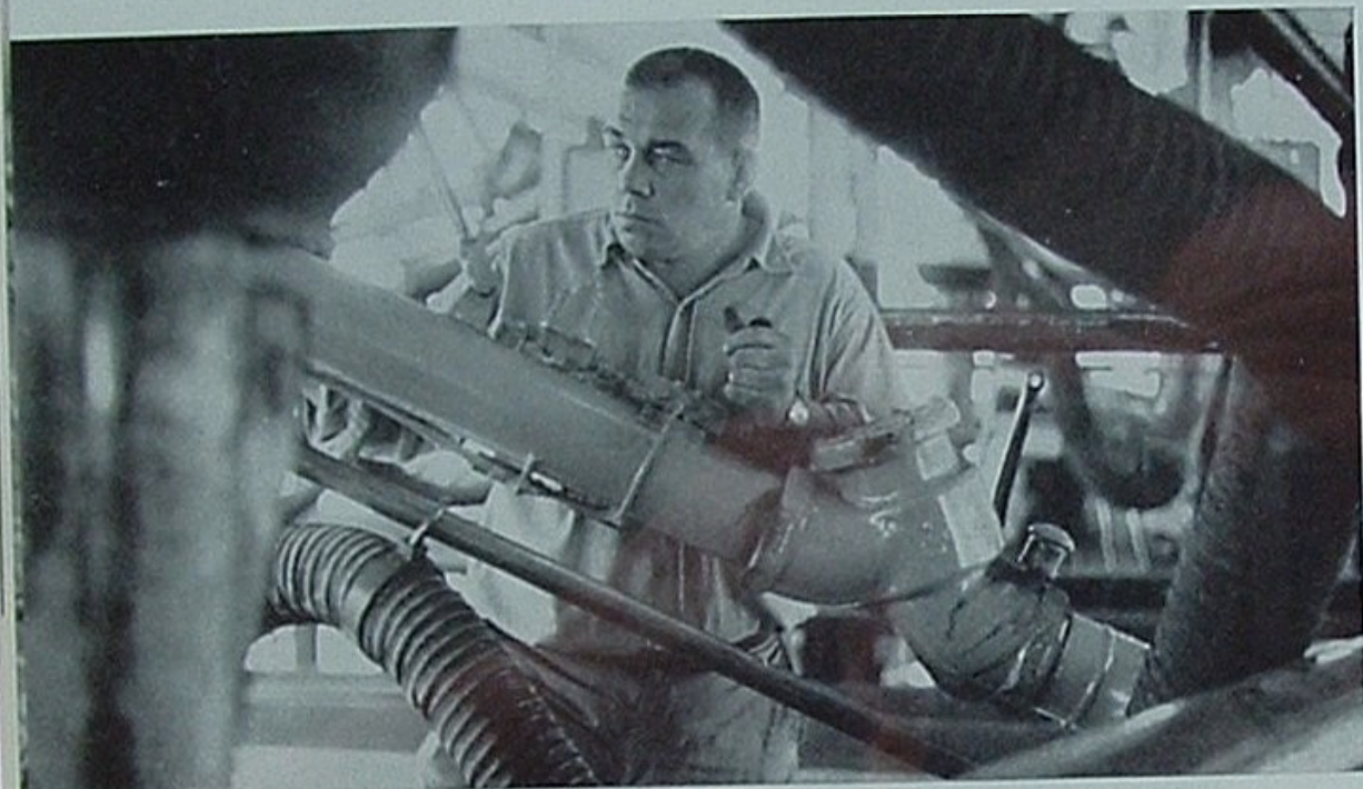
As loader Gay Wamre triggers gasoline into a transport compartment, rich gasoline vapors are vented out through flexible hose into recovery system.
