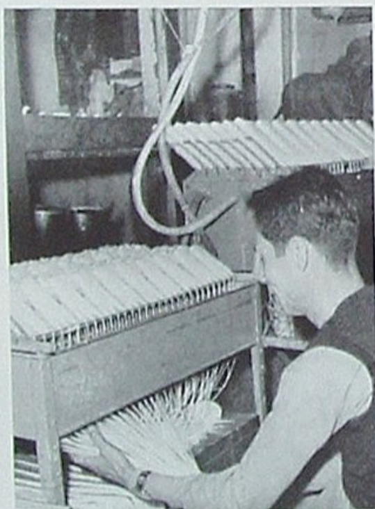
Standard candles for domestic use are molded 300 at a time via clever process.
