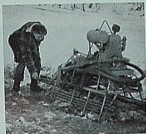
Shot-hole drilling equipment is designed to be pulled by tractor or lifted to location by the Sikorsky.
