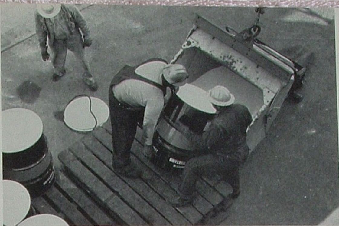
At Oleum Refinery, a barrel of the catalyst is dumped in hopper en route to the Reformer.
