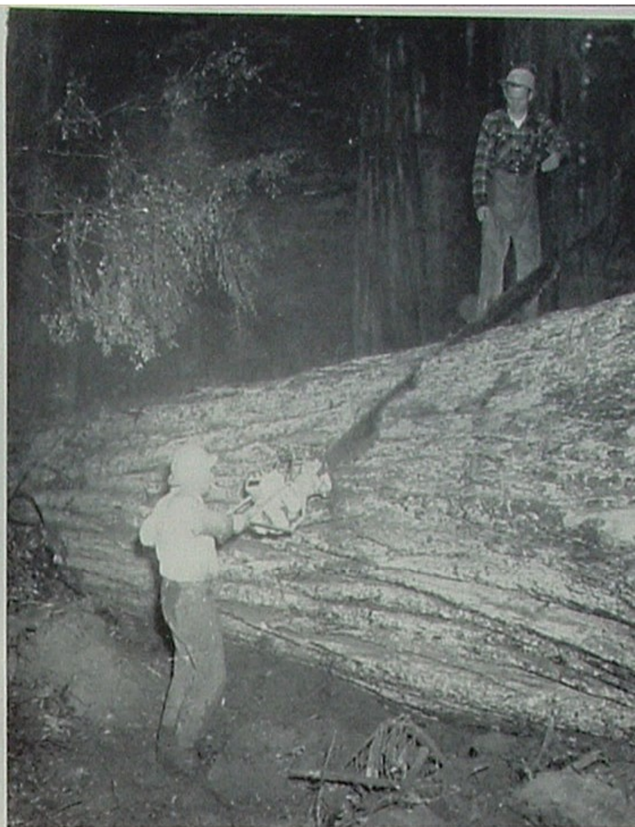
Bucking of the fallen giant into 24-foot lengths was done with a gasoline-powered chain-saw, nine-foot bar.
