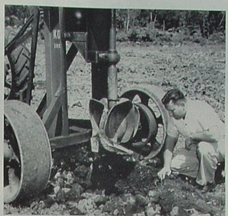
So impregnated with lava boulders is the volcanic slope of Mauna Loa that John Cross, orchard manager for Castle & Cooke, uses a special auger to drill holes for the nut trees.
