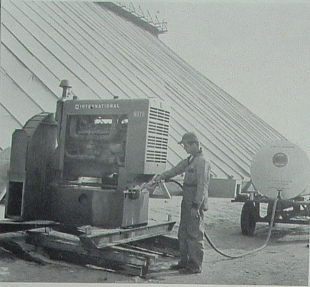
Gasoline-powered blowers circulate air through a 13,000-ton storage unit to aerate seed and prevent its deterioration.
