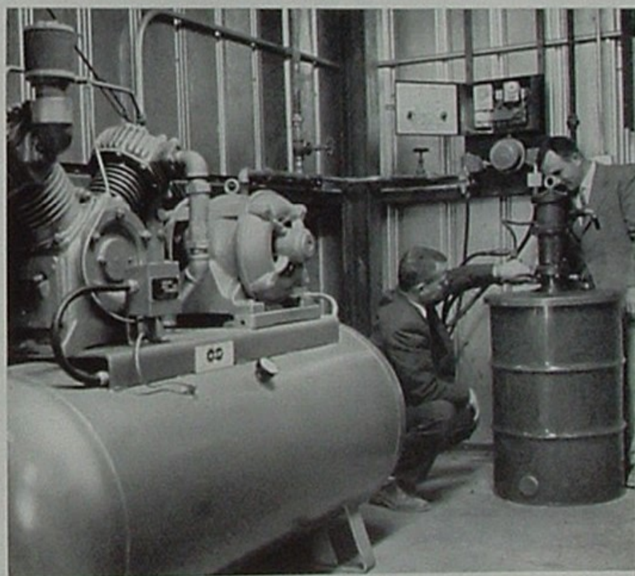
Union Oilers Mike Ryan and Pat McConnell of Fresno take studious interest in the plant's automatic lubrication system. Lubricants applied every 15 minutes via tubing, shown on delinter at left, have greatly increased the service life of bearings and machines.
