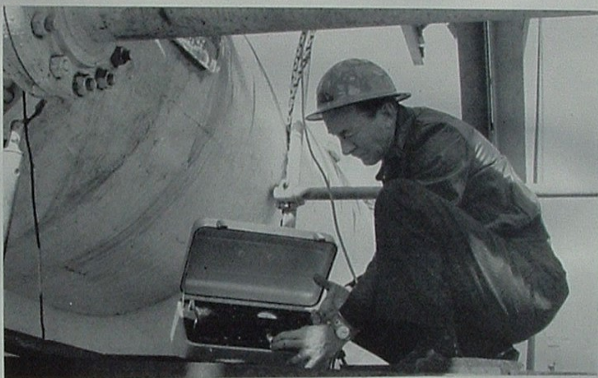
Bill Field uses a Corrosometer as a means of quickly measuring corrosion or the effectiveness of inhibitors.
