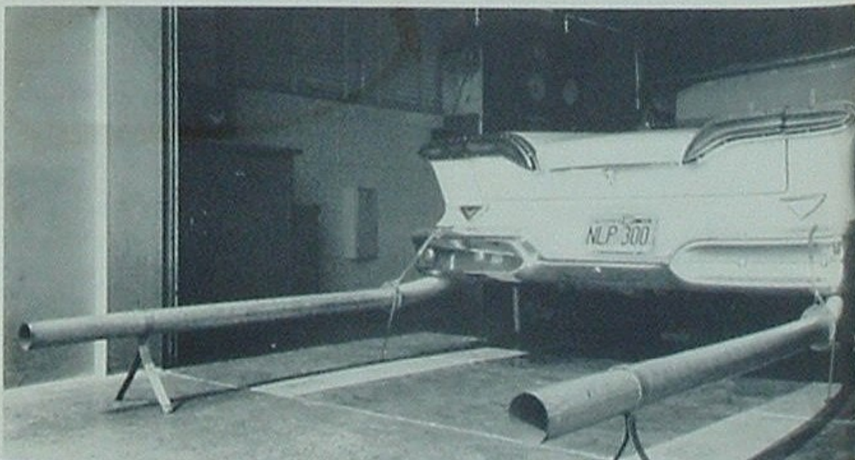
(Left) During road tests of clean-carburetor additives, cars were driven in daytime, researchers such as Bill Kent (left) and Jack Graham checked engines at night. (Below) Long pipes lead exhaust gasses from car undergoing octane tests at Research.
