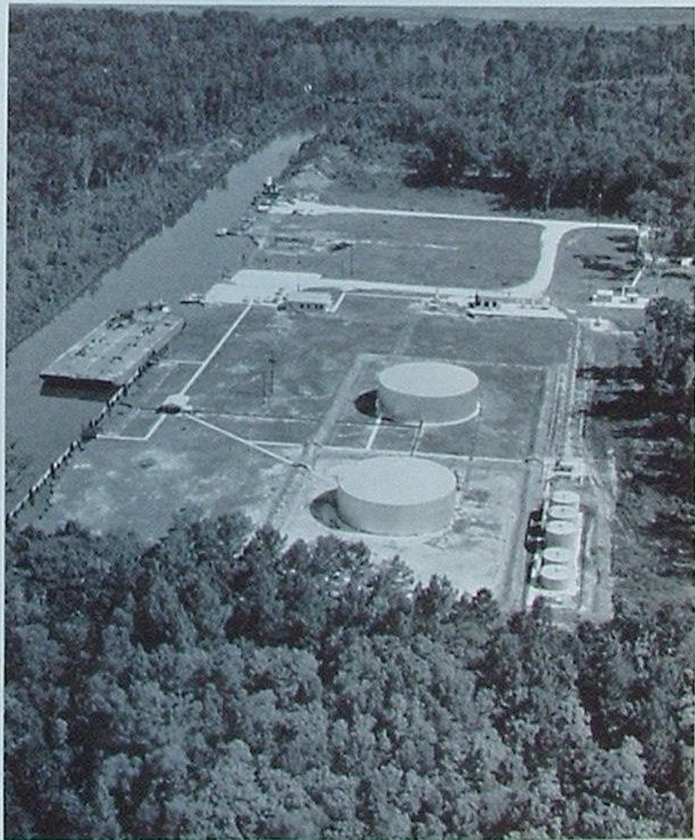
At this East Lake Palourde shipping point, condensate and heavier crude are stored for barge transport; natural gas, completely dry, enters pipeline of the transmission company.
