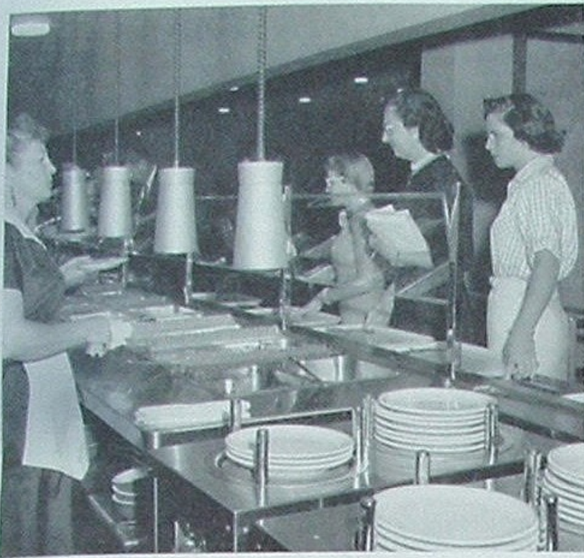
The problem of keeping air cool and food hot was solved by employee suggestion—electric heaters over serving trays.
