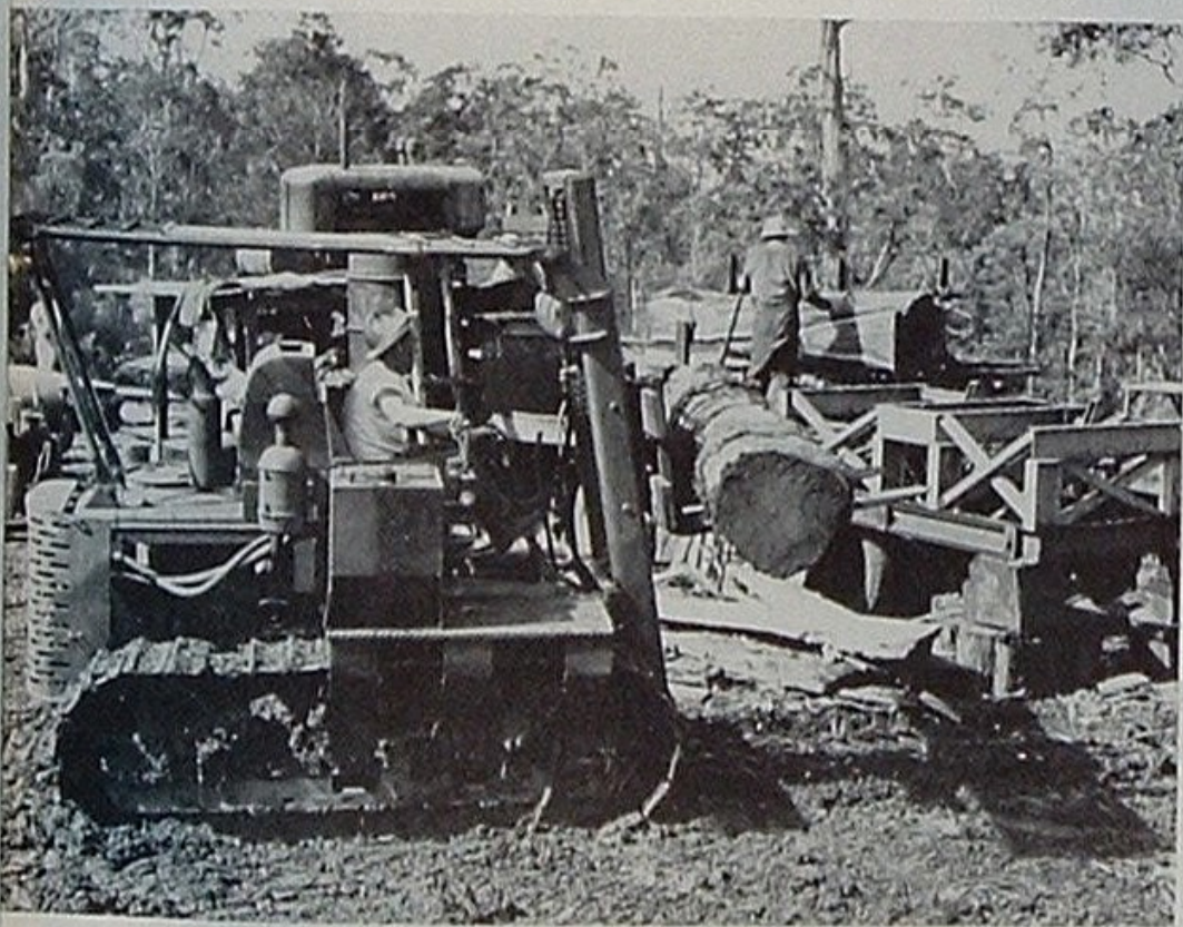
Portable milling equipment employed by Tropical Koa near the logging site eliminates hauling of waste down slopes of volcanic Mauna Loa.
