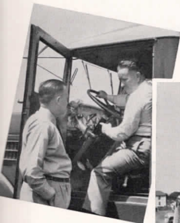
Right: This huge, Diesel powered Kenworth truck has a special spreader operated from the cab by air pressure.
