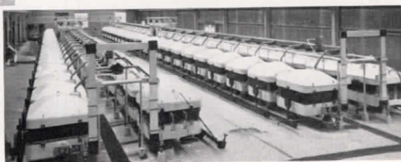
Right: This interior view of one of the cell houses shows the installation of a huge battery of electrolytic cells used to break down the common salt solution to form chlorine gas and caustic soda. The caustic soda solution is then concentrated and shipped by tanker and special rail tank cars to all manufacturing centers in the United States.
