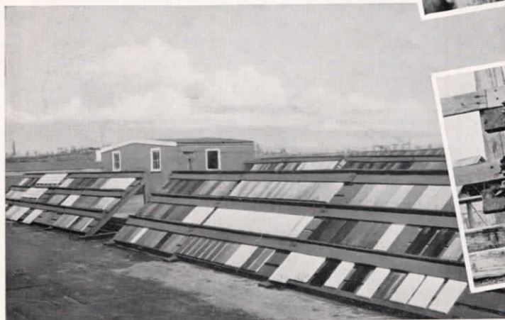
Above: Testing marine paints, duplicating conditions under which the paint will continually be used.
