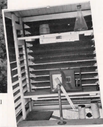
Below: Weather recording instruments are protected by a louvred housing.
