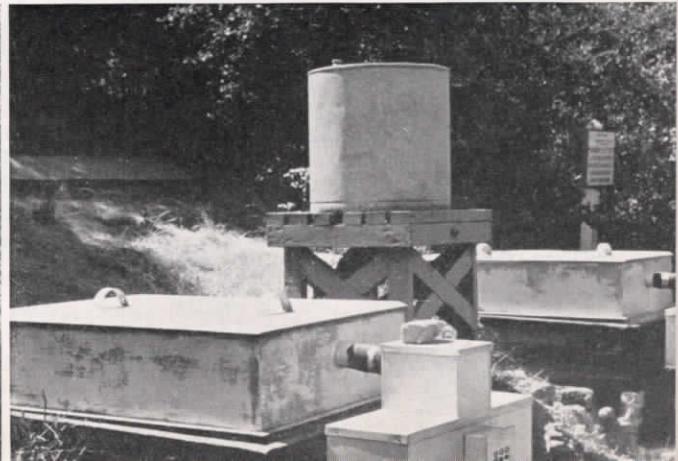
Tanbark Flat electric run-off and erosion recording devices developed to investigate the retarding influence of vegetation.
