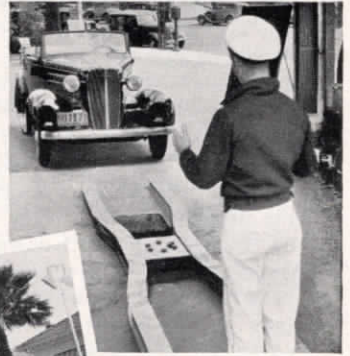
Above: Attendant guides motorist aboard pneumatic lift.
