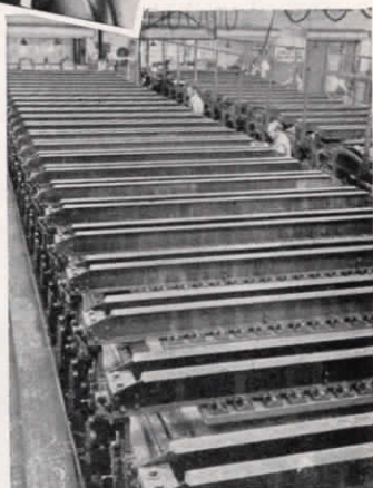
Right: The pattern printing machines are precision instruments which place each color in its proper position.
