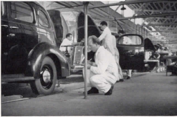
Above: First time the motor is actually operating on the line. Mechanic checks the performance.
