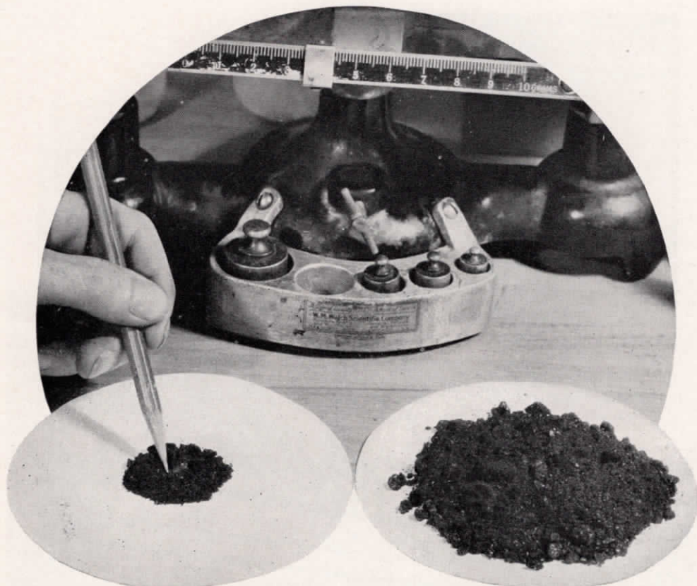
Above are shown relative quantities of carbon deposited by Triton (left) and a high grade eastern oil (right) in 7 days' operation of auxiliary Diesel engine on the tuna clipper "Reliance". When Triton was used, the deposition of carbon was only about 5% of former accumulations, and there was no indication of the sludging that had characterized the use of other oils.
