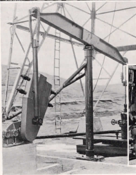
Left: Type of pumping equipment, powered by electric motor, used at Mt. Poso and, below, pump for circulating mud.
