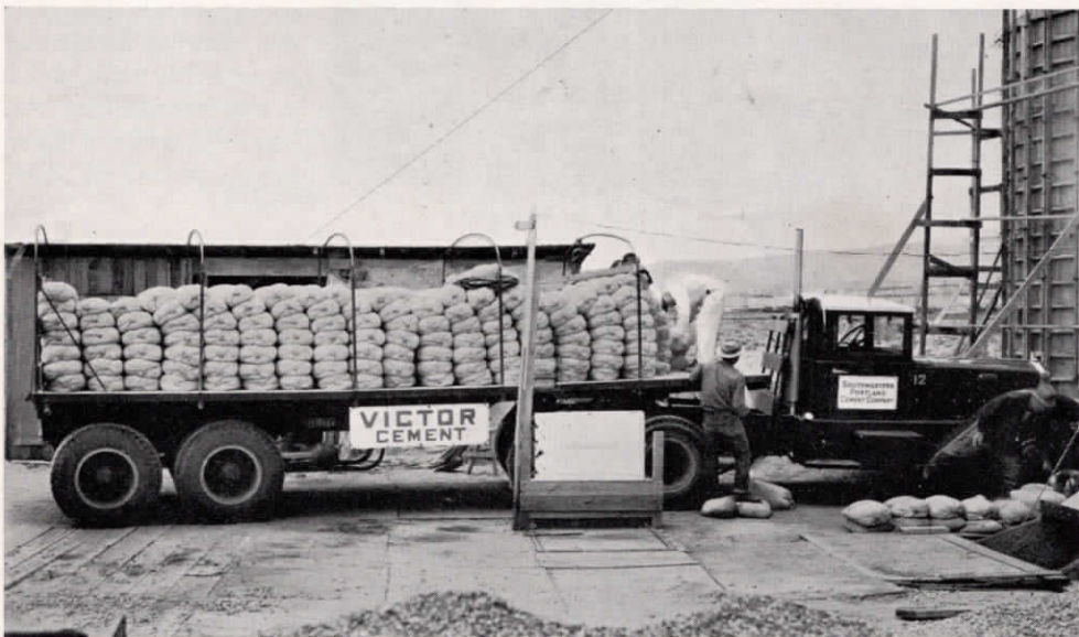
One of the large ten-wheel, semi-trailer Sterling tractors used by Southwestern Portland Cement Company, which is capable of transporting 400 sacks of cement in one load.
