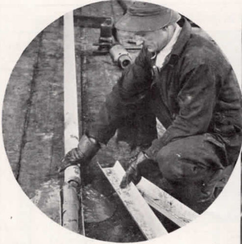
A core, taken with a regular formation coring device, is being removed from core barrel in the upper photograph, while at the right is core bit.
