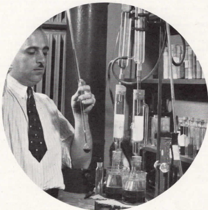
Dr. H. G. Reiber conducting test with Soxhlet Extractor in which he is extracting Pyrethrines from Pyrethrum flowers.
