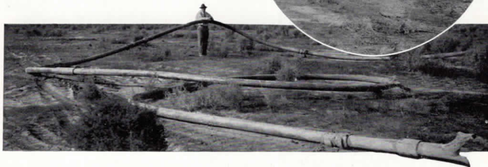
These photographs, taken by E. B. Noble, assistant chief geologist of the Union Oil Company, show what happens when a big gas well goes on a "bender." Stanley Wissler, paleontologist for the company, is examining the coiled drill pipe.
