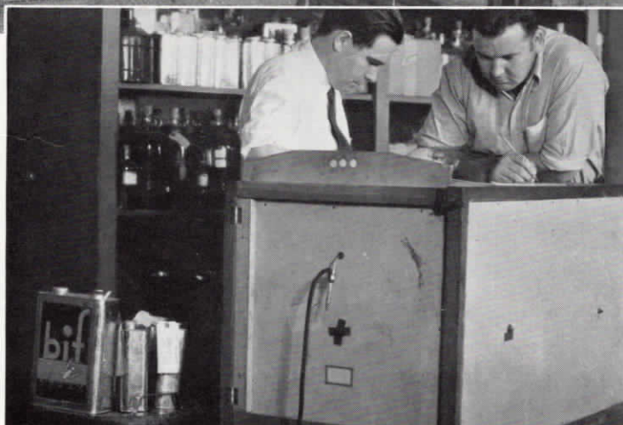
Trapping flies for the "Bif" test. In the circle, Dr. Jewel is shown placing fly cage in lethal chamber, and at the left he and an observer are charting the results of the "Biffing."
