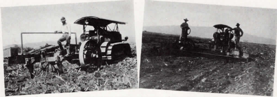
Sub-soiler, used to prepare field for planting, is shown on the left, while on the right, a field is being leveled preparatory to making furrows in which the cane is to be planted.
