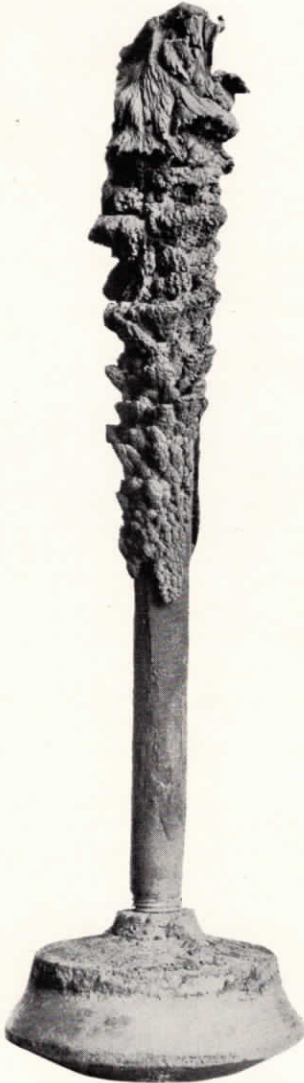
An Interesting Example of Carbon Deposition. This Frequently Occurs on the Thermometer Wells in a Liquid Phase Cracking Still. The Etching of the Carbon Surface is as Delicate and Beautiful as a Winter Frost Crystal.
