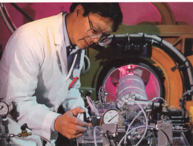
Top, a research chemist tests a catalytic process that converts natural gas to liquid transportation fuel. Above, a research technician uses a CAT scanner to monitor the flow of acid through a well core sample.
