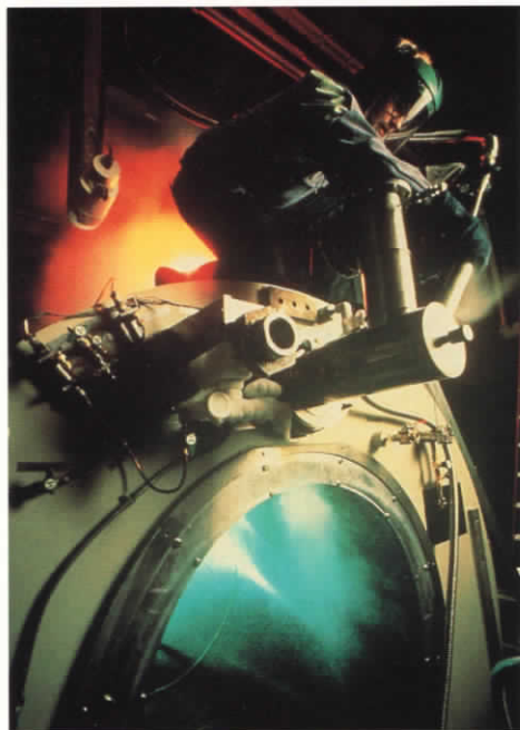
Left, a worker loads a magnetic resonance imaging machine with liquid helium. The superconducting magnets used in these advanced medical diagnostic devices are cooled by the product.
