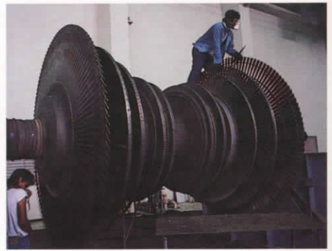
Right, a worker inspects portion of a turbine at one of the Bulalo field's three power plants. Below, workers fit a Tiwi steam pipe with new insulation.
