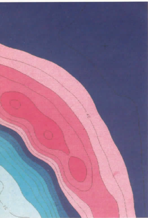
This computer generated oil saturation profile shows the projected course of a caustic waterflood through a reservoir that has been "watered out" by a secondary waterflood. The caustic flood (blue) moves away from an injection well, pushing an oil bank (pink) toward production wells.
