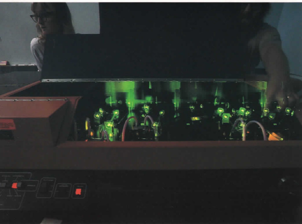
A portion of the Nd:YAG laser beam is diverted to provide the energy for the dye laser (Left).
