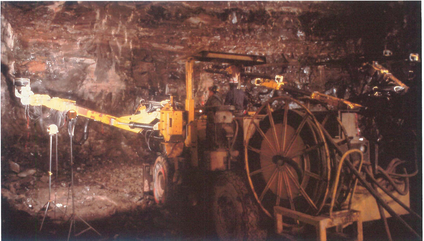
"Jumbo's," large self propelled hydraulic drills, bore holes ten feet into the mine face for explosives.
