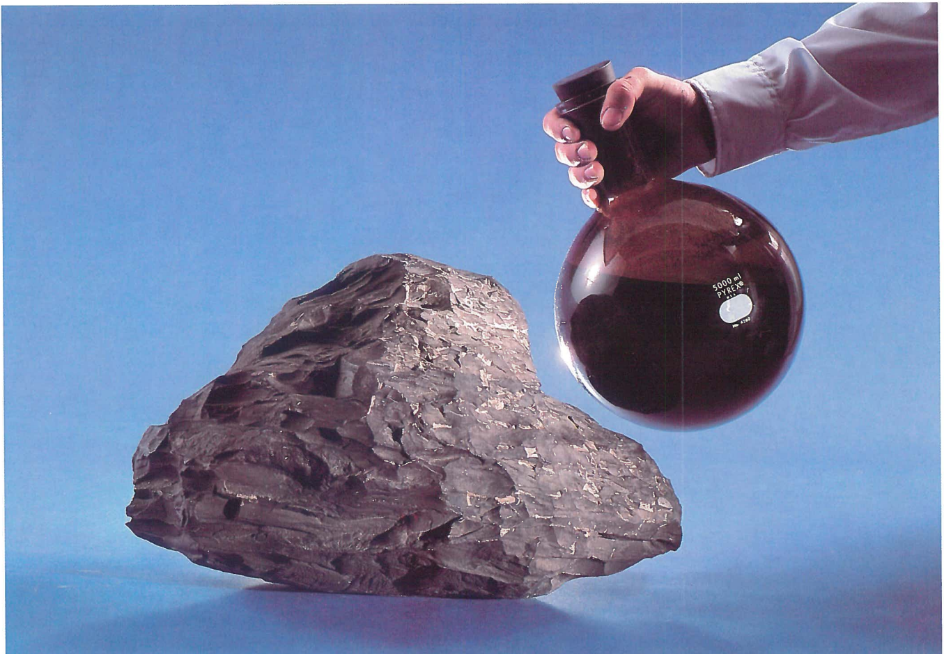
This piece of oil shale rock, weighing almost 59 pounds, will yield one gallon of shale oil when subjected to temperatures of 700 to 900 degrees.
